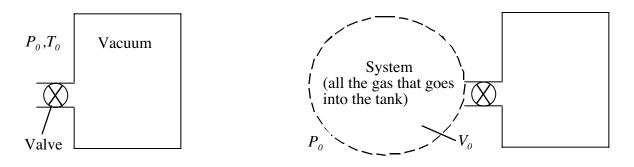
Figure 0-3: A transient problem—filling of a tank from the atmosphere
