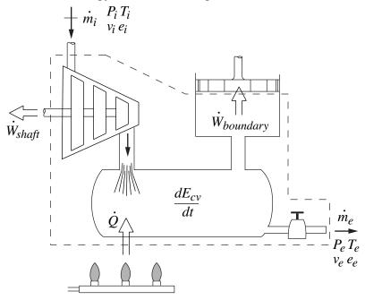
Figure 0-5: Schematic diagram illustrating terms in the energy equation for a control volume
