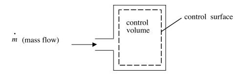
Figure 0-6: A control volume approach to the tank filling problem
