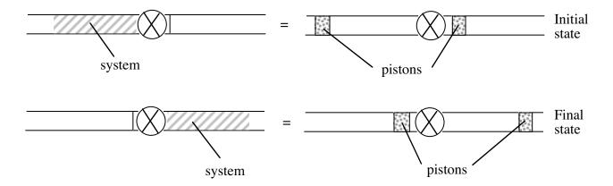
Figure 0-2: Equivalence of actual system and piston model
