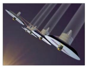
Figure 8. Separated Spacecraft Interferometer Example
