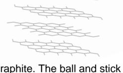
Graphite. The ball and stick model of graphite indicates the closely-packed nature of the carbon atoms. The layers of carbon in graphite are 335 pm apart, approximately twice as long as the C-C bond distance of 142 pm.
