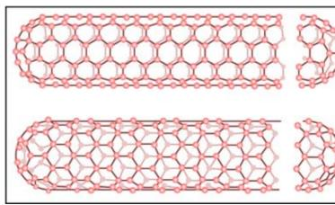
Carbon nanotube. The molecules vary in length from a few nanometers to a micrometer or more.
