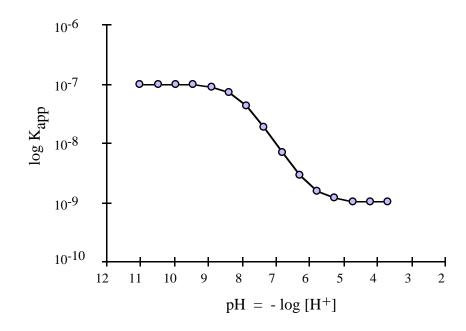
If this were experimental data, we could fit it to get  $pK_a$ 's for proton binding to the free protein ( $pK_a = -\log (K_3) = 6$ ) and to the complex ( $pK_a = -\log (K_2) = 8$ ).
