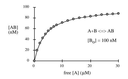
The shape of the equilibrium curve depends upon the reaction mechanism and can be used to decide between different equilibrium models.
