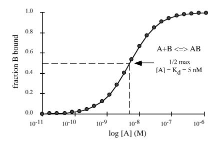
For any bimolecular reaction, 10% of B will be bound when  $[A] = K_d/9$  and 90% of B will be bound when  $[A] = 9K_d$ . Thus, 80% of the binding reaction occurs over a concentration range of about 80-fold in [A] centered around the  $K_d$ .
