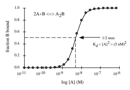
The Scatchard plot for this reaction is concave downward, which is diagnostic of a reaction showing positive cooperativity<sup>1</sup>. In this case, the cooperativity arises because A dimerizes in the bound  $A_2B$  complex.
