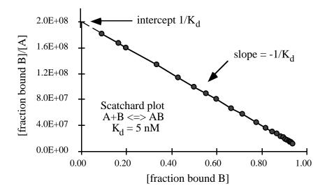
Hyperbolic binding curves and linear Scatchard plots are diagnostic of simple bimolecular reactions. Later on, we'll show that higher-order reactions such as  $2A+B \Leftrightarrow A_2B$  and  $3A+B \Leftrightarrow A_3B$  give Scatchard plots that are concave downward and binding curves with sigmoid shapes.
