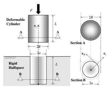
Deformable cylinder in a rigid halfspace.
