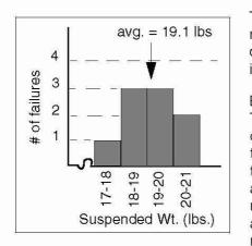
The results of your nine tests are shown at the left. The results cluster around 19/20 lbs which is quite surprising considering the sensitivity of this type of failure mode to imperfections.
