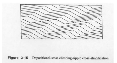
**4.2.11** The lamination produced when ripples move with a positive angle of climb is called climbing-ripple cross stratification. Examples with angle of climb so small that the contacts between sets are erosional (as in Figure 3-14) might be called *erosional-stoss* climbing-ripple cross stratification, and examples with angle of climb large enough for preservation of the full ripple profile (as in Figure 3-15) might be called *depositional-stoss* climbing-ripple cross stratification.
