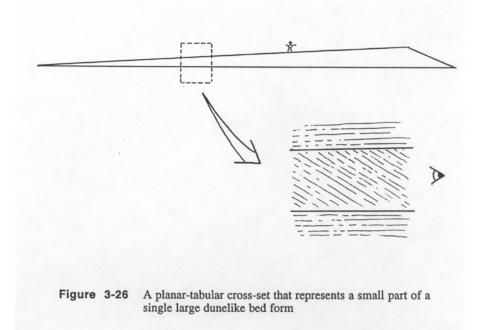
**4.3.6.4** In a situation like that shown in Figure 3-26, there's also the problem of *whether the full height of the dune is preserved*. You might find features at the upper surface of the cross-set that gives evidence of its having been the exposed upper surface of a dune, like superimposed smaller bed forms. Although that's not foolproof, it would suggest strongly that the dune was not eroded or shaved off by a later strong current after its own driving current ceased.
