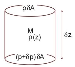
Figure 2: Hydrostatic balance
