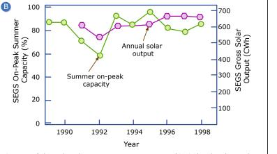
Output of the solar electric generating systems (SEGS) solar thermal power plants in California (data are from ref 9). The SEGS plants had significant reductions in on-peak capacity and total output following the eruption of Mt. Pinatubo.
