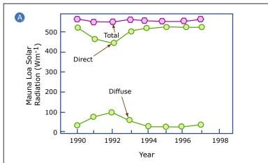
Sunlight measured at Mauna Loa. The reduction in direct sunlight and increase in diffuse sunlight following the eruption of Mt. Pinatubo in 1991 are readily apparent. The reduction in total sunlight was much smaller.
