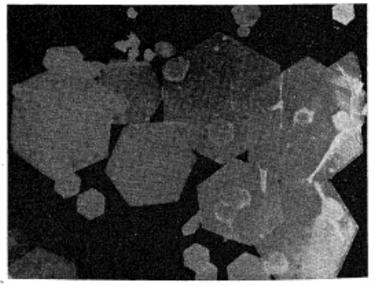
FIG. 3. Lead-iodide crystals formed in cooling water.
