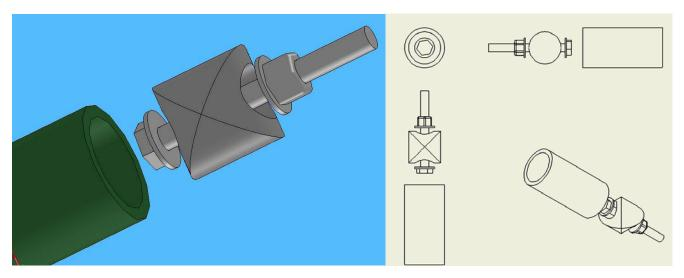
**Figure 14: Second Alignment Assembly.** This assembly requires only six pieces and can be easily tightened before positioning within the pylon. We plan to test the effectiveness of larger versions of the assembly this summer.
