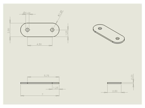
**Figure 4: Larger Knee Linkage.** This linkage was created from a piece of sheet steel using a band saw, drill press, and power sander. This linkage is placed on the front right side of the knee when viewed head on, as shown in Figure 6.
