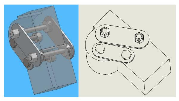
Figure 10: Completed Assembly for Multiple Linkage Knee. This assembly includes two high-density polyethylene blocks, two steel linkages, four bolts, and four lock nuts. The pieces to be manufactured are described in Figures 4,5,8, and 9. Note that two out of eight holes are countersunk, and that the design currently includes only three linkages. We will be investigating the effects of adding another linkage or damper in the same location this summer.
