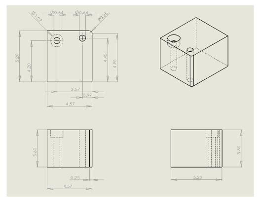
Figure 9: Lower Portion of Multiple Linkage Knee. Shown here is a three section view of our latter prototype's lower half. It is the same as that for the first prototype, except it contains two fewer countersunk holes.
