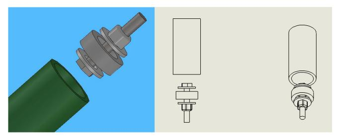
Figure 11: Initial Alignment Assembly. Shown here is the completed assembly for the initial knee alignment system. It is created from a ring of plastic, two washers, and a nut and bolt.
