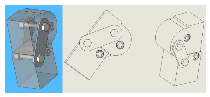
Figure 6: Completed Assembly for Single Linkage Knee. This assembly includes two high-density polyethylene blocks, two steel linkages, four bolts, and four lock nuts. The pieces to be manufactured are described in Figures 2 through 5.
