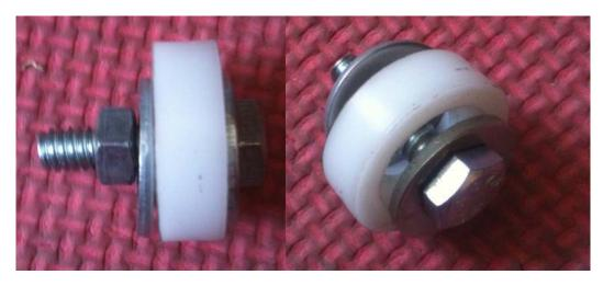
**Figure 11: Initial Alignment System.** In the alignment system pictured here, a short ring of Delrin is used to support a moveable bolt, which is to be screwed into the top of a prosthetic knee joint. The alignment system is then tightened in the desired position and fastened to the end of a pylon.
