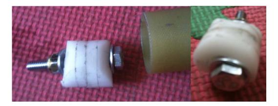
Figure 12: Second Alignment System. This alignment system, machined from a single piece of one inch tube stock, allows for both linear vertical and angular positioning.
