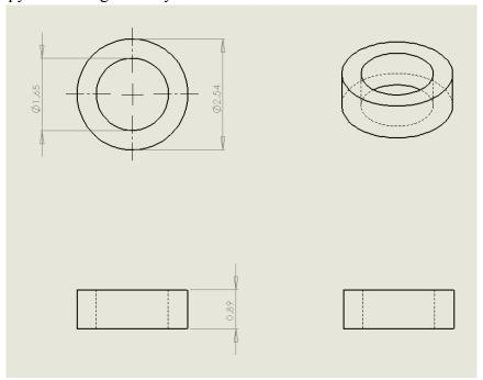
Figure 12: Three Angle View of Alignment Ring. The above drawing shows the construction of our initial alignment ring prototype. Dimensions, shown in centimeters, should be proportionally scaled according to the necessary size of the alignment system. The alignment ring can be manufactured using a drill press in one inch stock, as well as in a water jet from thick sheet plastic.
