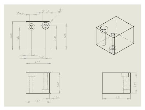
Figure 3: Bottom Portion of Single Linkage Knee. Shown here is a three-section view of the knee's bottom portion. The accompanying physical part was manufactured via the same processes as the knee's upper portion.
