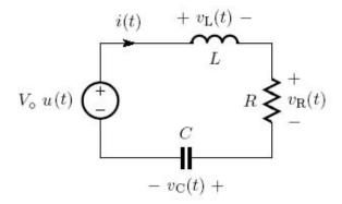
Figure 1: A step-driven series RLC circuit.
