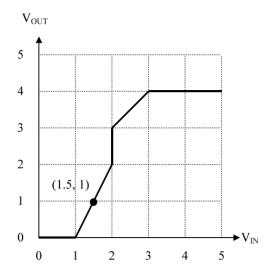
Your job is to choose a single set of signaling thresholds  $V_{ol}$ ,  $V_{il}$ ,  $V_{ol}$ , and  $V_{il}$  to be used with both devices to give the best noise margins you can. Recall that the VTC can touch the edge of the forbidden regions but not pass through those regions. Fill in your answers below, together with the resulting noise margins. You'll get partial credit for anything that works with nonzero noise margins; for full credit, maximize each of the noise margins.
