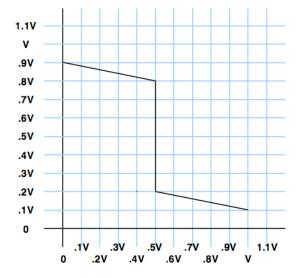
(B) What is the maximum noise immunity that can be realized using this device as an inverter, with an appropriately chosen signaling specification?
