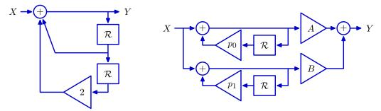
It is possible to choose coefficients for the block diagram on the right so that the systems represented by the left and right block diagrams are "equivalent". 1
