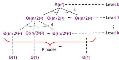
This recursion tree recursively branches 4 ways until it reaches the first level  $k$  that contains  $P$  nodes. Each worker then serially executes the computation under a distinct level- $k$  node, which the recursion tree models with 1-way branching after level  $k$ .
