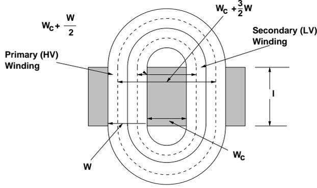
Figure 3: Winding Length Estimate
