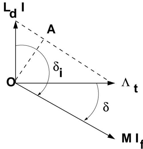
Figure 1: Vector Diagram for Torque Theorem Proof
