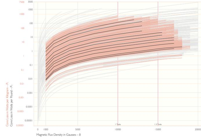
— Total core loss curves for this material, 50 through 2000 hertz
