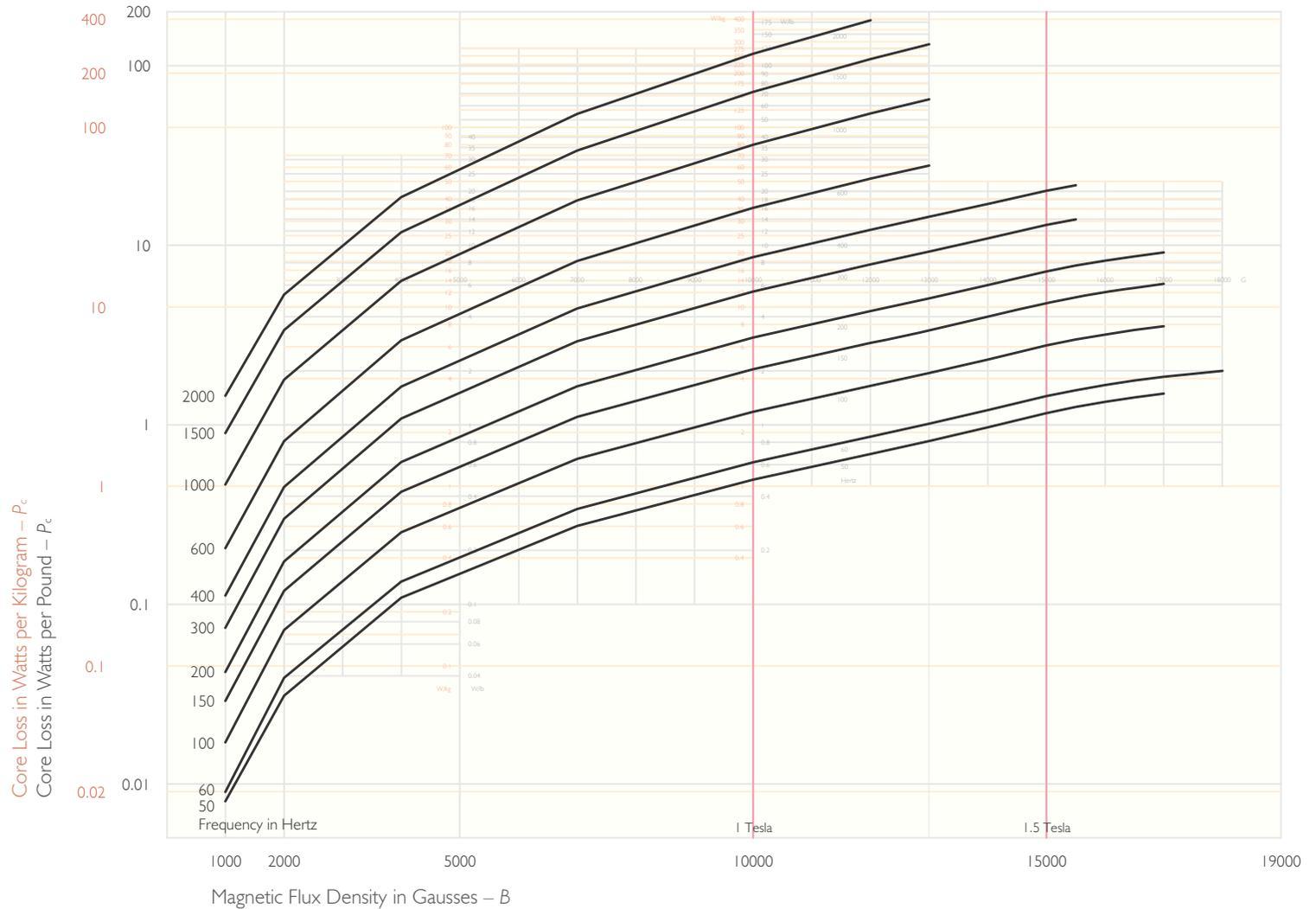
Typical total AC core loss of as-sheared .014 inch (.36 mm, 29 gauge) Di-Max M-19 fully processed cold-rolled non-oriented silicon steel. See core loss data page for data values. Curves developed from previously unpublished information provided by AK Steel, 2000. Chart prepared by EMERF, 2004.
