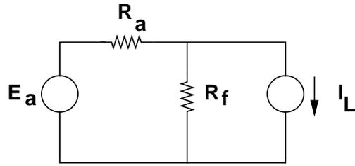
Figure 6: Dynamo Circuit
