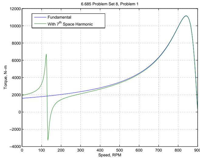
Figure 2: Torque-Speed with Seventh Harmonic
