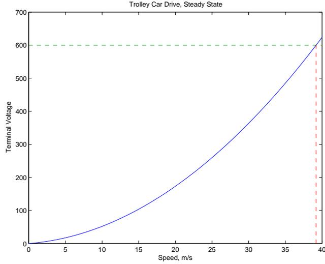
Figure 3: Voltage required vs. speed
