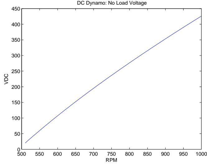
Figure 5: No Load Voltage
