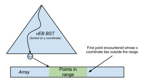
Figure 6: A high level description of the datastructure which supports 2 sided range queries using only linear space.
