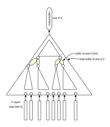
Figure 1: Memory layout for K-funnel sort.
