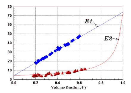
Figure 4: Rule-of-mixtures predictions for longitudinal  $(E_1)$  and transverse  $(E_2)$  modulus, for glass-polyester composite  $(E_f = 73.7 \text{ MPa}, E_m = 4 \text{ GPa})$ . Experimental data taken from Hull (1996).
