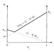
Figure 6: Strength of unidirectional composite in fiber direction.
