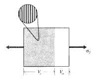
Figure 3: Loading perpendicular to the fibers.
