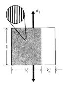
Figure 2: Loading parallel to the fibers.
