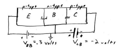
The E-B junction is forward-biased. The C-B junction is reverse-biased.  $\Rightarrow$  We are in the forward-active regime.  $I_E\approx I_C>>I_B.$
