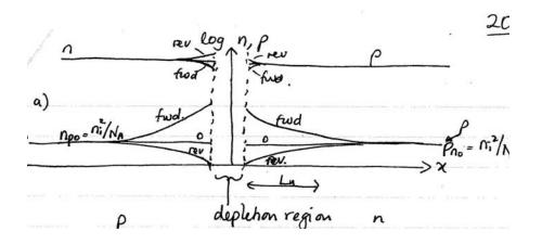
depletion region, decays away with characteristic length  $L_n$  (10s of  $\mu$ m) slight reduction of electron concentration near depletion region of n side. Reverse Bias: e collected from p side, pins n = 0. (Very slight increase in n on the n side.)
