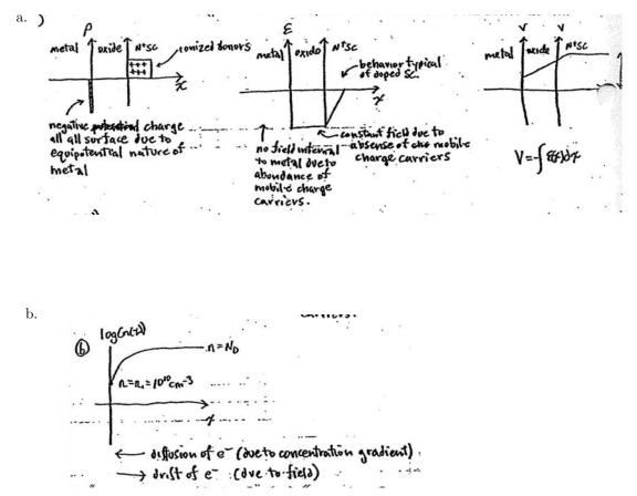
"Is x in equilibrium?"  $\Leftrightarrow$  "Is the fermi level flat within x?" Within the semiconductor the Fermi Level remains flat, meaning there is no tendency for charge to flow in either direction. The semiconductor, considered separately from the rest of the system is "in equilibrium" within itself. The additional band bending due to the applied MOS voltage is then considered to create a sort of new built-in voltage, similar to what we saw in a pn junction.
