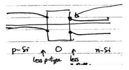
Like MOS; the S/C - oxide band offsets are fixed, same for all doping levels. Equilibrium - Band bending casuses depletion near each interface.
