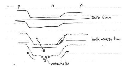
Note: Putting EB in fwd bias means a large current already flows through  $E \rightarrow C$ , so the light-generated carriers would not add much to this.
