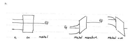
Material masked in black is oxide  $(SiO_2)$  $V_G$  negative: initially electrons depleted from S/C, eventually goes into inversion (becomes p type). Metal gate has depletion of electrons close to interface.  $V_G$  positive: electrons accumulate in S/C and also in metal near interface.
