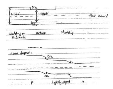
(The cladding thickness doesn't matter too much but you need the active layer to be thin enough so we can get a high density of photons. Also need to avoid dislocations forming due to misfit with substrate. Length of device governed by where you want the nodes due to cavity resonance.) Typical for slc laser
