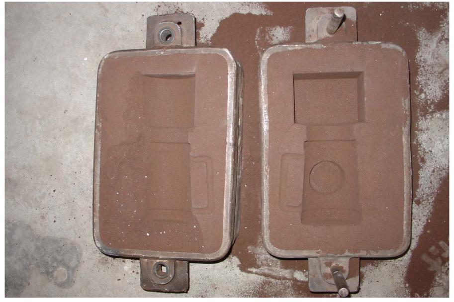
The pattern is removed from the sand flasks, leaving a cavity in the shape of the pattern mug. Metal can then be poured into this cavity.
