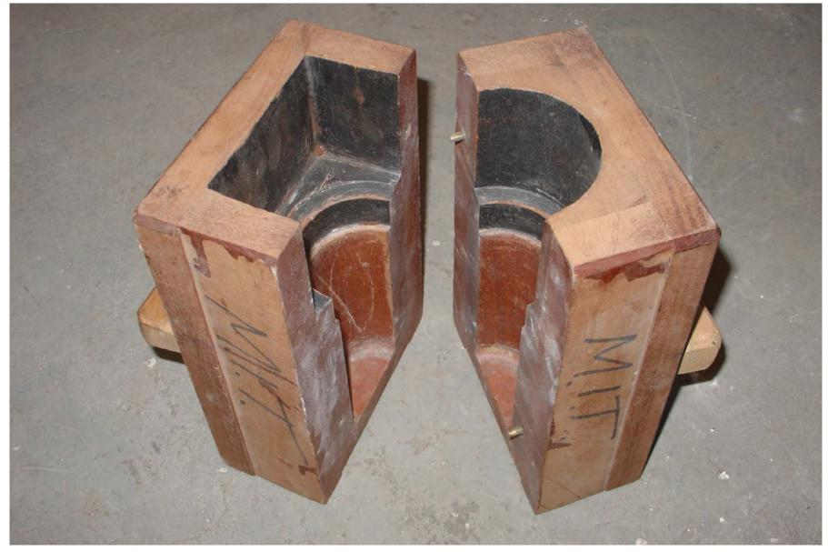
Since the mug needs to be hollow, a core must be inserted into The mug-shaped cavity, to displace volume. Above is a "core box," used as a mold to make cores.
