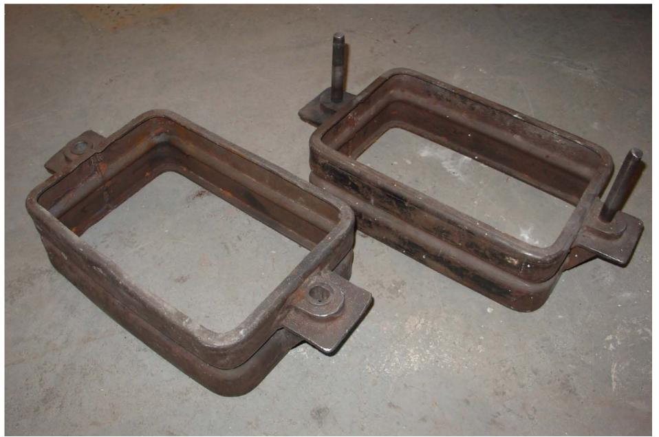
Sand casting flasks -- cope & drag -- that form the sand molds
