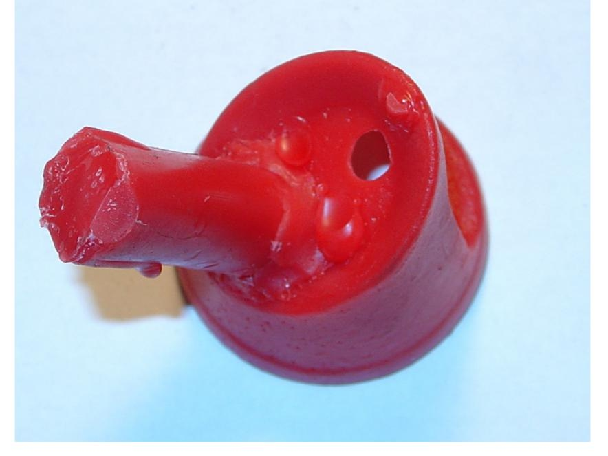
A finished wax, as removed from the rubber mold
