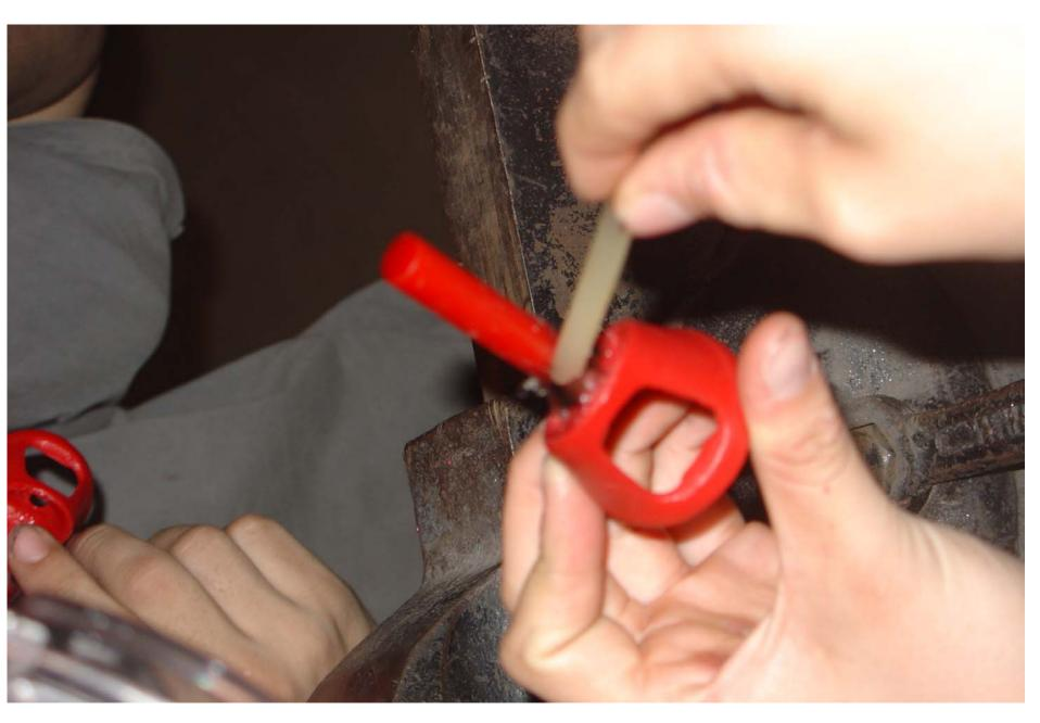
Attaching gates to wax objects using "sticky wax" as adhesive
