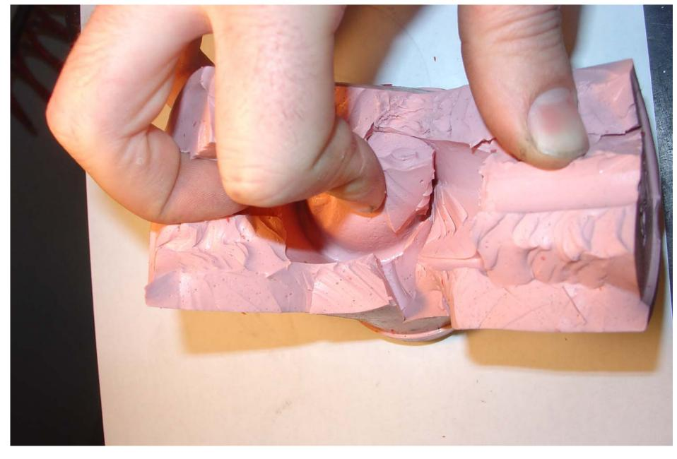
The inside of the bottle-opener rubber mold, showing the cavity left by the molded object.
