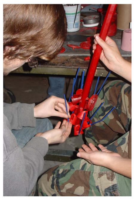
Adding vents to objects to allow air to escape during casting
