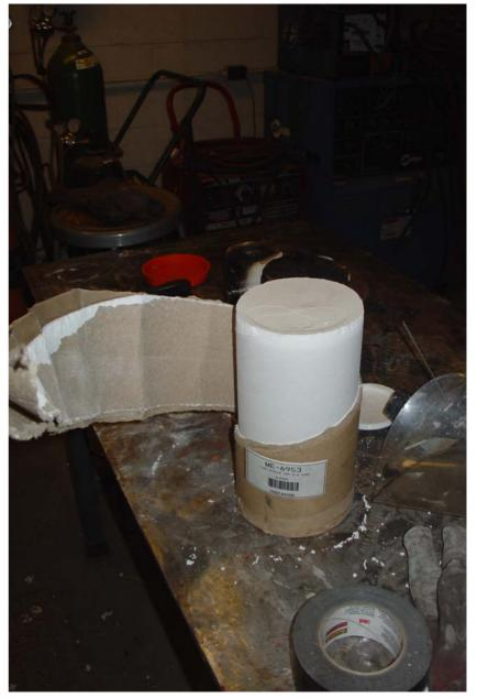
Removing cardboard tube in preparation for wax burnout
