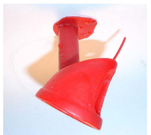
The most crucial part of lost-wax casting is producing a quality wax model. The metal you cast will be a very close replica of your original wax. Even fingerprint-level detail can be transferred from wax to metal. This wax is a wall-mount bottle opener.
