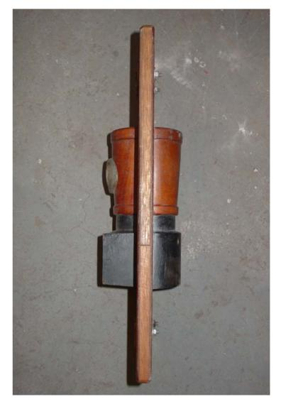
Above is a sand casting pattern. This is a model of what is cast
