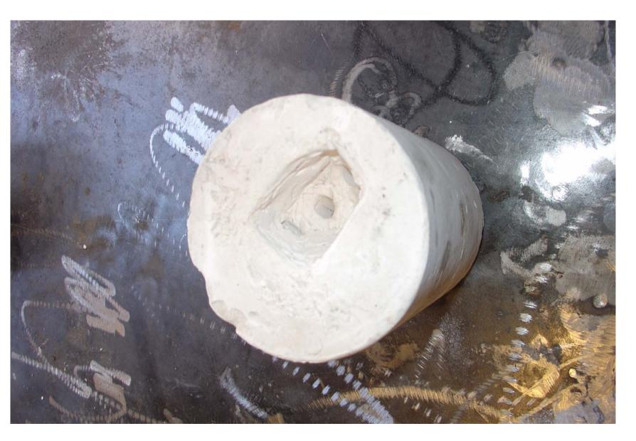
De-waxed ceramic mold ready for pouring Once wax is removed, molds are fired/sintered in a furnace
