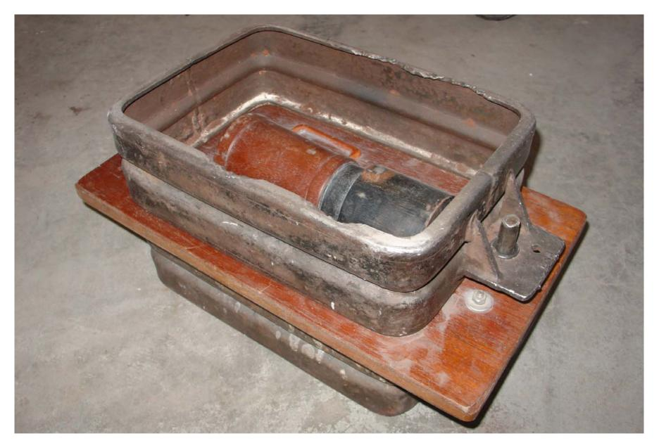
The pattern is placed between the flasks, and foundry sand is rammed into the cope and drag, around the pattern form
