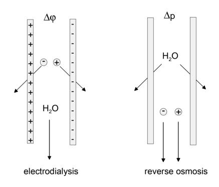
irreversible energy loss proportional to ion transport  $(E_{irr} = z_i F \Delta C_i U V)$
