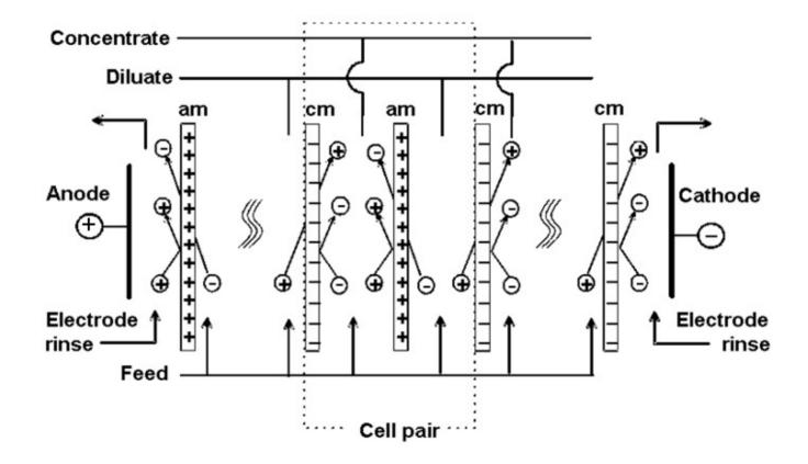
ions are removed from a feed solution and concentrated in alternating cells a cation and an anion-exchange membrane, and a diluate and concentrate cell form a cell pair
