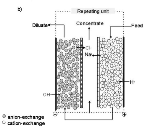
good removal of weak acids but electrode reaction by-products and cation leakage maximum achievable resistance < 10 M  $\Omega$  cm
