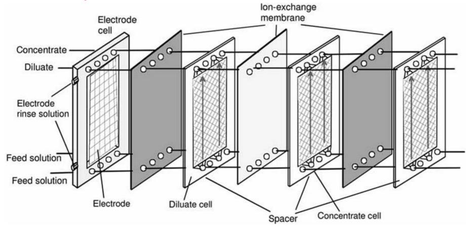
an electrodialysis stack is composed of 100 to 400 cell pairs between electrode compartments
