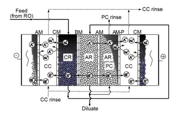
good removal of weak acids, repeating units can be stacked between electrodes, maximum achievable resistance < 10 M  $\Omega$ cm
