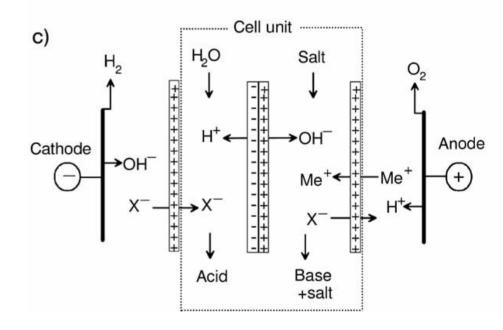
production of a pure acid and a base-salt mixture
