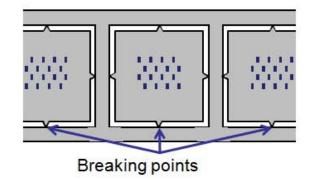
Top: membranes are patterned to break at determined points. The frame carries multiple membranes for a repeatable and automated process.
