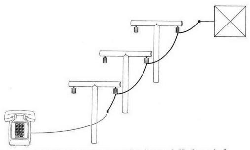
Figure 10.1. A telephone is connected to the central office by a pair of wires.
