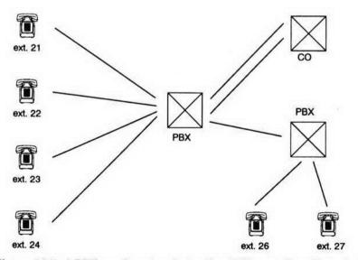
**Figure 10.7.** A PBX may have trunks to other PBXs as well as the central office, providing private telephone networks.
