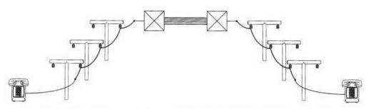
Figure 10.2. Telephones connected through trunk lines between two central offices.
