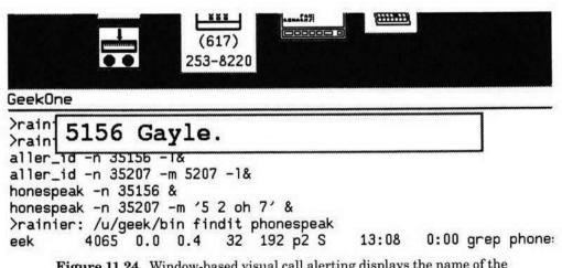
Figure 11.24. Window-based visual call alerting displays the name of the calling party.
