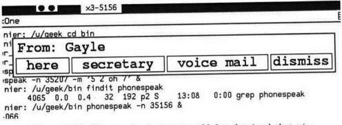
Figure 11.25. When routing buttons are added to the visual alert window, the called party can dynamically forward calls when working in another office.
