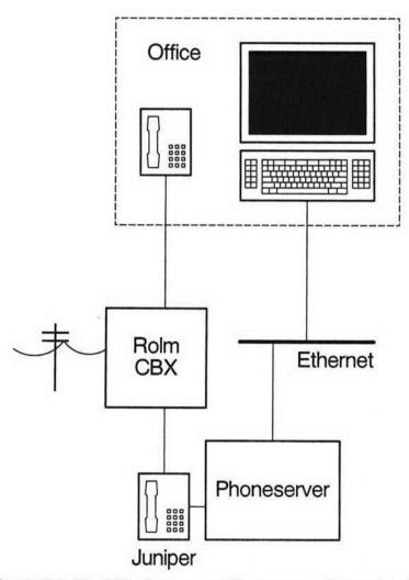
**Figure 11.8.** The I.S.I. phoneserver utilizes a personal computer with a specialized interface card to control the PBX. Workstations make requests of this server over a local area network. (From Schmandt and Casner, "Phonetool: Integrating Telephones and Workstations." Reprinted with permission from *IEEE Global Telecommunications Conference* © 1989, IEEE.)
