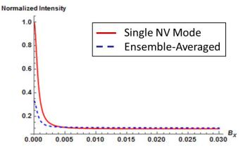
**Figure 9:** A plot demonstrating the effect of the transverse field on the observed signal when the system is biased around the excited state LAC. Clearly the observed signal approaches a steady value for  $B_x \gtrsim .002T$ . In generating this plot  $B_z = .05T$  and  $\Gamma = 10$ .
