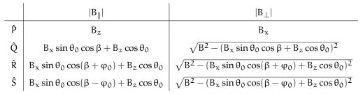
**Table 2:** The parallel and perpendicular projections of an external magnetic field  $\vec{B} = B_x \hat{x} + B_z \hat{z}$  onto the 4 possible defect axes. The angles  $\theta_0$ ,  $\beta$  and  $\phi_0$  are defined in the text.
