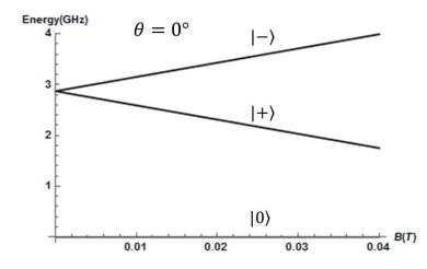
Figure 2: A depiction of the Zeeman splitting of the triplet ground state.
