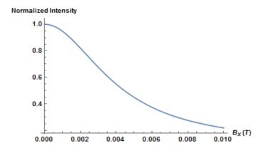
Figure 3: The normalized PL intensity as a function of the transverse magnetic field amplitude. The parallel projection onto the defect axis is held constant at  $B_z = .03T$ .
