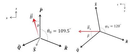
Figure 4: (Left) The tetrahedral geometry to be considered. The tetrahedral angle is 109.5° and  $\rho$  is the angle between  $\vec{B}$  and  $\hat{z}$ . (Right) The tetrahedral geometry projected into the transverse plane. The angle of symmetry is 120° and  $\beta$  is the offset of the tetrahedron with the x-axis, which is defined along the transverse field component.
