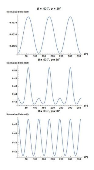
Figure 5: Rotation profiles of the observed signal within the x-y plane.  $\rho$ , the angle between  $\vec{B}$  and  $\hat{z}$ , increases from top to bottom from 20° to 85° to 90°. For all, |B| = .03T and  $\Gamma$  is set to 10. The intensities are normalized to the  $\rho = 0^{\circ}$  intensities.
