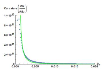
**Figure 11:** (Blue) A plot of the curvature of the signal profile evaluated at  $B_z = .052T$ and  $\Gamma = 10$  as a function of  $B_x$ . (Green) A fitted curve  $\frac{\partial^2 S}{\partial B_z^2}\Big|_{.052} = \frac{586038}{(B_x - .0005T)^2}$  to extract the leading order dependence of the signal curvature upon  $B_x$ .
