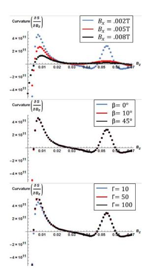
Figure 10: A series of plots depicting the dependencies of the signal curvature on  $B_x$  (Top),  $\beta$  (Middle) and  $\Gamma$  (Bottom). Clearly, a change in the transverse field magnitude is the dominant cause for changes in the observed signal curvature. It is therefore proposed that by monitoring the changes in the signal curvature the transverse perturbation magnitude can be determined.
