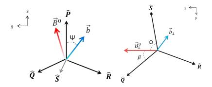
**Figure 8:** The geometry of the perturbing magnetic field.  $\Psi$  is the angle between the perturbing field and the z-axis, and  $\Omega$  is the angle between the perturbing field and the x-axis.
