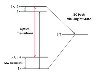
Figure 1: The seven level model in the absence of an external magnetic field, consisting of the ground state and excited state triplets and a metastable singlet. Only spin-conserving radiative transitions and non-radiative transitions to the metastable state are considered.
