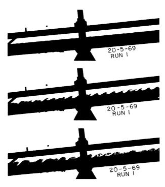
Figure 8.6 The breakdown of an interface in a shear flow to produce an array of Kelvin-Helmholtz billows. (Thorpe, 1971.)
