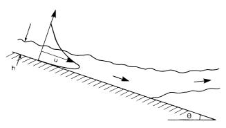
Figure 8.14 Sketch of a steady gravity current on a slope; the edge shown represents the level of most rapid variation of density. The outer part of the velocity profile sketched is linear, and so is the density profile at this level. (Ellison and Turner, 1959.) In stratified surroundings, the plume leaves the slope at a depth given by equation (8.48).
