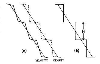
Figure 8.4 Discontinuous profiles produced by mixing, from initially linear density and velocity distributions. In (a) the final profiles, different for density and velocity, correspond to a constant gradient Richardson number everywhere, and (b) is the simpler model of homogeneous layers and thin interfaces used to derive (8.26).
