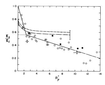
Figure 8.12 The ratio of transport coefficients for magnesium  $(K_4)$  and potassium  $(K_2)$  measured by Griffiths (1979) across a diffusive interface, with heating below. The ratio of molecular coefficients  $K_4/K_2 \approx 0.60$ , and the upper curves are Griffiths's theoretical predictions.
