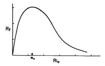
Figure 8.5 Schematic relation between the flux Richardson number Rf and the overall Richardson number  $Ri_0$  for experiments on mixing across a density interface. (After Linden, 1979.) The maximum of the curve corresponds to the "equilibrium" condition.
