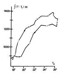
Figure 8.3 The heat content in the surface layer as a function of surface temperature  $T_0$  at ocean weather station Echo. (After Gill and Turner, 1976.) The reference temperature  $T_r$  is the mean of the temperature at 250 m and 275 m depth, and the months are marked along the curve.
