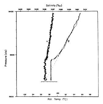
Figure 8.13 Salinity (S) and potential temperature ( $\theta$ ) profiles measured by Armi and Millard (1976) in the middle of the Hatteras Abyssal Plain. The dashed line indicates that the structure could have formed by mixing up a stratified region above the bottom.
