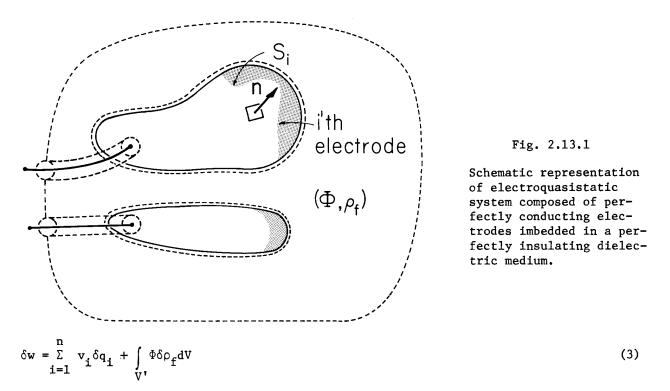
The volume V' is the volume excluded by the electrodes. Note that the reference electrode is not included in the summation, because the electric potential on that electrode is, by definition, zero. The work required to place a free charge at its final position correctly accounts for the polarization, because the polarization charges induced in carrying the free charges to their final position are reflected in the potential.
