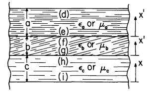
Fig. 2.20.1. Convention used to denote surface variables.
