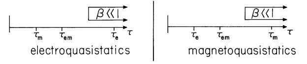
Fig. 2.3.1. Possible relations between physical time constants on a time scale T which typifies the dynamics of interest.
