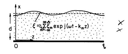
Fig. 7.12.1. Planar region is excited from transverse boundary at  $x = d + \xi$ . Longitudinal boundary conditions typically represent a load at  $z = \ell$  and a source at z = 0.
