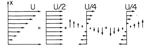
Fig. 7.14.3. Plane shear flow divided into translation, rotation and strain-rate flow.
