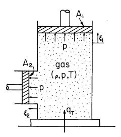
Fig. 7.22.1. Schematic view of lumped-parameter thermodynamic subsystem.
