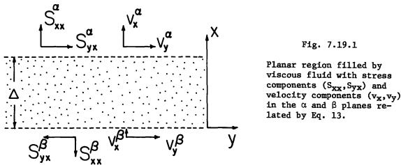
For perturbations having the form Re  $A_v(x)$  exp j( $\omega t - ky$ ), Eq. 1 requires that the complex amplitude,  $A_v(x)$ , satisfy a fourth-order differential equation that has two solutions familiar from the incompressible inviscid fluid model of Sec. 7.9,
