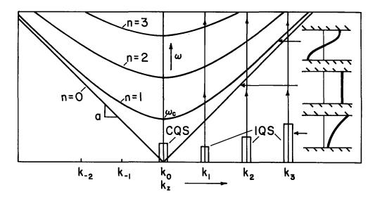
Fig. 7.12.2. Regions of  $\omega$ -k<sub>z</sub> plane characterize x dependence of response to transverse drive of each Fourier mode as driving frequency is raised.
