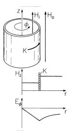
**Fig. 10.3.2** Circular cylindrical conducting shell with external axial field intensity  $H_o(t)$  imposed. The response to a step in applied field is a current density that initially shields the field from the inner region. As this current decays, the field penetrates into the interior and is finally uniform throughout.
