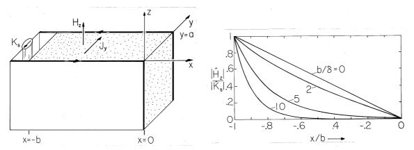
Fig. 10.7.2 (a) One-dimensional magnetic diffusion in the sinusoidal steady state in the same configuration as considered in Sec. 10.6. (b) Distribution of the magnitude of  $H_z$  in the conducting block of (a) as a function of the skin depth. Decreasing the skin depth is equivalent to raising the frequency.
