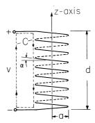
Fig. 10.1.1 Side view of long inductor having radius a and length d.
