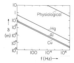
Fig. 10.7.3 Skin depth as a function of frequency.
