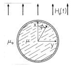
Fig. 10.4.2 Circular cylindrical conducting shell filled by insulating material of permeability  $\mu$  and surrounded by free space. A magnetic field  $H_o(t)$  that is uniform at infinity is imposed transverse to the cylinder axis.
