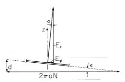
Fig. 10.1.2 With the wire from the inductor of Fig. 10.1.1 stretched into a straight line, it is evident that the slope of the wire in the inductor is essentially the total length of the coil, d, divided by the total length of the wire,  $2\pi aN$ .
