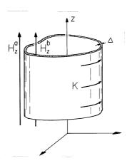
**Fig. 10.3.1** A thin shell having conductivity  $\sigma$  and thickness  $\Delta$  has the shape of a cylinder of arbitrary cross-section. The surface current density K(t) circulates in the shell in a direction perpendicular to the magnetic field, which is parallel to the cylinder axis.
