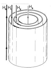
Fig. 10.5.2 Example of an axial field configuration composed of coaxial conducting shells of infinite axial length. When an exterior field  $H_o$  is applied, currents circulating in the shells tend to shield out the imposed field.
