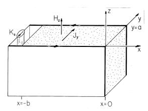
**Fig. 10.6.1** A block of uniformly conducting material having length b and thickness a is sandwiched between perfectly conducting electrodes that are driven along their edges at x=-b by a distributed current source. Current density and field intensity in the block are, respectively, y and z directed, each depending on (x,t).
