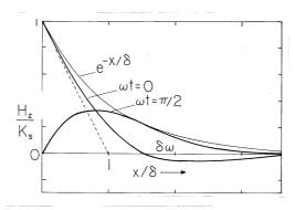
Fig. 10.7.1 Magnetic diffusion wave in the sinusoidal steady state, showing envelope with decay length  $\delta$  and instantaneous field at two different times. The point of zero phase propagates with the velocity  $\omega\delta$ .
