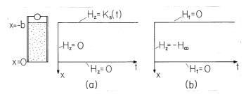
**Fig. 10.6.2** Boundary and initial conditions for one-dimensional magnetic diffusion pictured in the x-t plane. (a) The total fields at the ends of the block are constrained to be equal to the driving surface current density and to zero, respectively, while there is one initial condition when t=0. (b) The transient part of the solution is zero at the boundaries and satisfies the initial condition that makes the total solution assume the current value when t=0.
