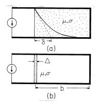
Fig. 10.7.5 Perfectly conducting  $\supset$ -shaped conductors are driven by a distributed current source at the left. The magnetic field is shielded out of the region to the right enclosed by the perfect conductors by: (a) a block of conductor that fills the region and has a thickness b that is large compared to a skin depth; and (b) a sheet conductor having a thickness  $\Delta$  that is less than the skin depth.
