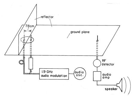
Fig. 12.7.3 Demonstration of phase shift on radiation pattern.
