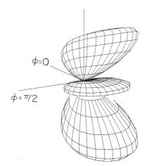
Fig. 12.4.8 Radiation pattern for two center-fed wire antennas, quarter-wave spaced, 90 degrees out-of-phase, each having length  $3\lambda/2$ .
