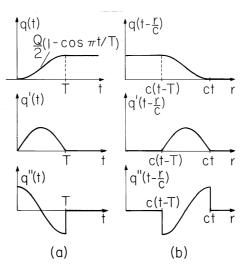
**Fig. 12.2.5** (a) Time dependence of the dipole charge q(t) as well as its first and second derivatives. (b) The radial dependence of the functions needed to evaluate the dipole fields resulting from the turn-on transient of (a) when t > T.
