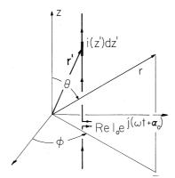
Fig. 12.4.2 Line current distribution as source of radiation field.
