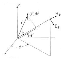
**Fig. 12.4.1** Incremental current element at  $\mathbf{r}'$  is source for radiation field at  $(r, \theta, \phi)$ .
