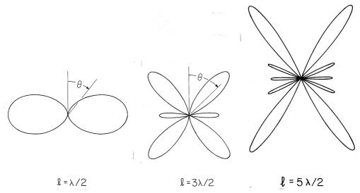
Fig. 12.4.4 Radiation patterns for center-fed wire antennas
