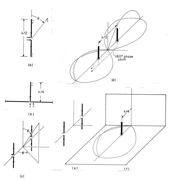
Fig. 12.7.2 Equivalent image systems for three physical systems.
