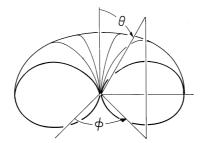
**Fig. 12.2.7** Radiation pattern of short electric dipole, shown in the range  $\pi/2 < \phi < 3\pi/2$ .
