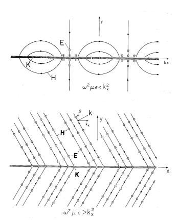
Fig. 12.6.4 TE fields induced by traveling-wave source in the y=0 plane.
