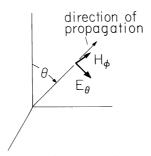
Fig. 12.2.4 Far fields constituting a plane wave propagating in the radial direction
