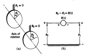
Fig. 2.2.3 An angular position source: (a) physical; (b) schematic.
