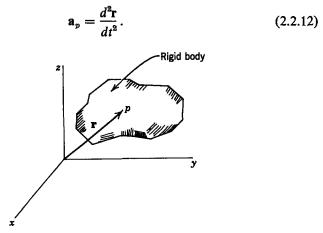
Fig. 2.2.12 Geometry for analyzing the translation of a rigid body.
