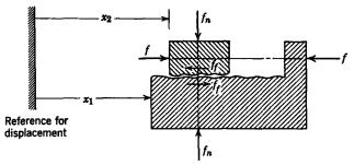
Fig. 2.2.8 Coulomb friction between members in contact.
