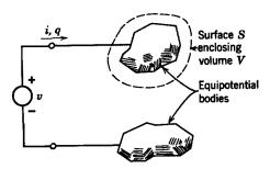
Fig. 2.1.6 A simple electric field system.
