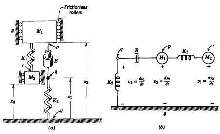
Fig. 2.2.17 Mechanical system and its network diagram: (a) system; (b) mechanical equivalent circuit.
