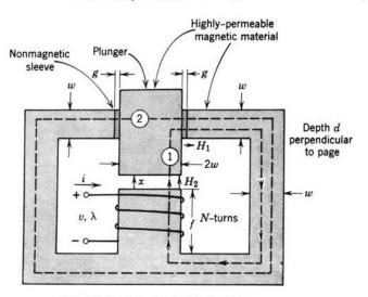
Fig. 2.1.2 A magnetic field system.
