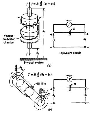
Fig. 2.2.7 Mechanical dampers: (a) translational system; (b) rotational system.
