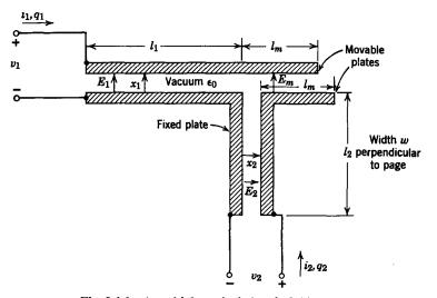
Fig. 2.1.8 A multiply excited electric field system.
