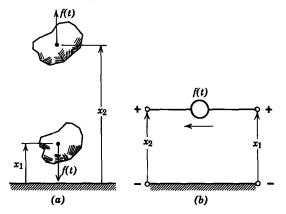
Fig. 2.2.2 A force source: (a) physical; (b) schematic.
