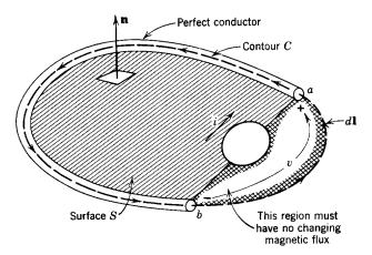
Fig. 2.1.1 Configuration for defining terminal voltage.
