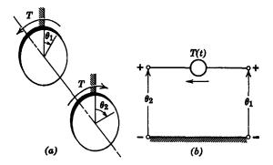
Fig. 2.2.4 A torque source: (a) physical; (b) schematic.
