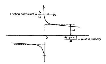
Fig. 2.2.9 Typical coulomb friction characteristic.
