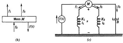
Fig. 2.2.15 System showing forces at a node: (a) system; (b) free body diagram of mass M; (c) circuit.
