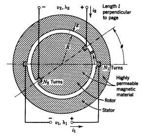
Fig. 2.1.3 Doubly excited magnetic field system.
