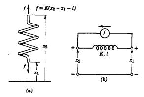
Fig. 2.2.5 A linear ideal spring for translational motion held in equilibrium by a force f: (a) physical system; (b) circuit.
