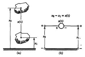
Fig. 2.2.1 A position source: (a) physical; (b) schematic.
