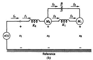
Fig. 2.2.18 One-dimensional model of auto suspension: (a) system; (b) equivalent circuit.
