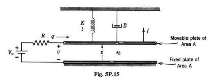
plate. The capacitor plates are excited by a constant voltage source in series with a resistance R. Neglect fringing fields. The voltage  $V_o$  is adjusted so that a stable, static equilibrium occurs at  $X_o = 0.7l$ . With the system at rest at this equilibrium position, a small step of mechanical force f is applied:  $f = Fu_{-1}(t)$ . In all of your analyses assume that the perturbations from equilibrium are small enough to allow use of linear incremental differential equations.
