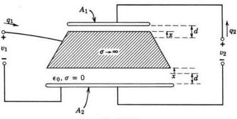
5.18. The central plate of a three-plate capacitor system (Fig. 5P.18) has one mechanical degree of freedom, x. The springs are relaxed in the equilibrium position x = 0 and fringing can be neglected. For a long time the system is maintained with the central plate fixed at x = 0 and the switch closed. At t = 0 the switch is opened and the center plate is released simultaneously.
