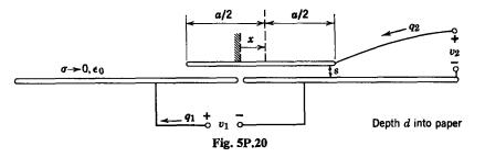
(b) Now the top plate is insulated from the lower plates after a charge  $q_2 = Q$  has been established. Also, the potential difference between the lower plates is constrained by the voltage source  $v_1 = V_0$ . Find a hybrid energy function  $W''(V_0, Q, x)$  such that
