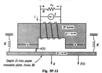
system is designed to provide linear operation about an equilibrium where the coil is excited by a constant current *I*. The plate is constrained at each end by springs that exert no force when x = 0.
