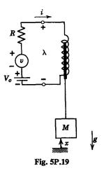
(b) With v(t) = 0, the current produced by  $V_o$  holds the mass M in static equilibrium at  $x = x_o$ . Write the linearized equations of motion for the perturbations from this equilibrium that result because of v(t).
