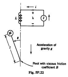
approximately by the expression  $L = L_o(1 + 0.2 \cos \theta + 0.05 \cos 2\theta)$ , where  $L_o$  is a positive constant. The coil is excited by a constant-current source I at a value such that  $I^2L_o = 6Mgl$  with no externally applied forces other than gravity g.
