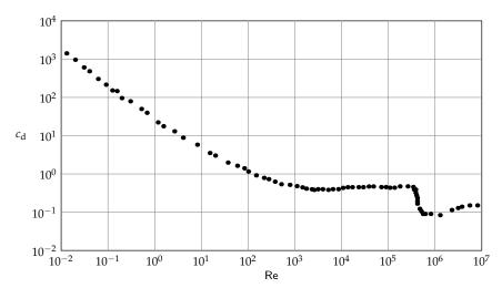
Like the drag coefficient for the cone, the drag coefficient for a sphere is almost constant as the Reynolds number varies from 3500 to 7000. The drag coefficient holds constant even throughout the wider range 2000...3  $\times$  10<sup>5</sup>. Around Re  $\approx 3 \times 10^5$ , the drag coefficient falls by a factor of 5, from 0.5 to roughly 0.1. This drop is the reason that golf balls have dimples (you will explain the connection in Problem 7.24).
