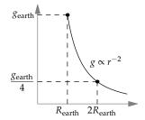
the gravitational acceleration falls from  $g_{\text{Earth}}$  to  $g_{\text{Earth}}/4$ . The graph shows that g(2R) is smaller than g(R); unfortunately, the scaling is hard to extract from these points or from the curve.
