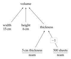
Now we propagate the values to the root. The two bottommost leaves combine to tell us that the thickness of one sheet is  $10^{-2}$  centimeters. This thickness completes the tree's second layer. In the second layer, the three nodes tell us that the volume of a dollar bill—the root—is 1 cubic centimeter.
