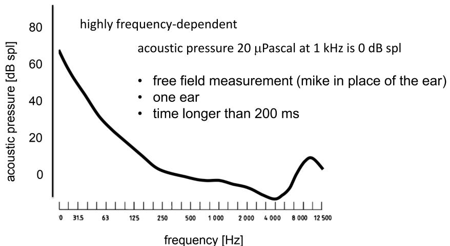
when signals are applied in in both ears, threshold for each is  $\Theta_{\rm B} = \Theta_{\rm M} / 2$  (signals integrate)
