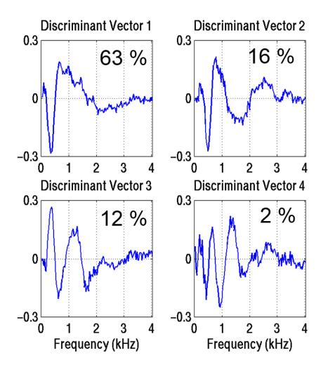
Spectral resolution of LDAderived spectral basis is higher at low frequencies
