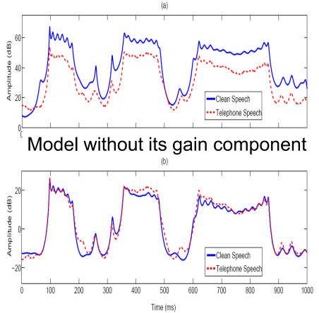
Ignoring FDPLP model gain makes the representation invariant to linear distortions introduced by the communication channel.
